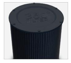
**360° MULTI LAYER FILTER** The 360° filter consists of a fine mesh prefilter, true HEPA filter, and activated carbon filter. Equipped with RFID intelligence for an easy filter change. Includes a premium textile cover.
